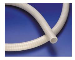
**Construction:** Platinum Cured silicone in compliance with FDA 21 CFR 177.2600, FDA-BfR part XV from Germany, and USP Class VI. Polyester reinforcement with stainless steel wire narrow pitched encased inside the hose.
