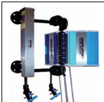
LevelMax unit for high pressure service (up to 3000 PSI (200 Bar)), including our Simpliport® Bicolor type water gage glass. The high pressure design for application pressures up to 3000 PSI (200 Bar) include chain wheel actuated water gage valves and flanged connections to the water gage.
