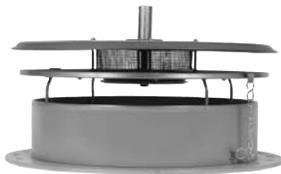
The pressure relieving cover is designed to lift only far enough to flow its rated capacity should high tank pressure be encountered then reseal automatically when the tank pressure is reduced. The webs on
