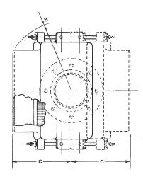
Note: 2" unit has a single flame arresting grid. 3" 4", 6" and 8" units have two flame arrester grids
