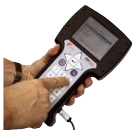
Figure 1. The CVA can be configured using a device with Bluetooth wireless technology such as a PDA or PC, alternatively a typical instrument shop HART communicator can be used.
