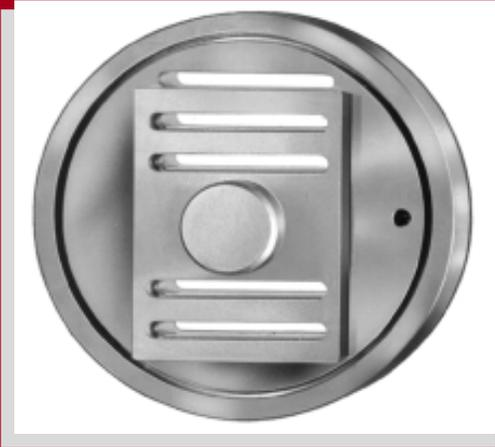
*Sliding gate seats are made up of a disc and plate, both slotted with openings that align to allow the required flow to pass through the orifices.*
