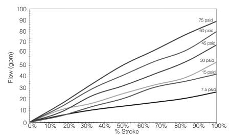
% STROKE VS FLOW (1-1/2" MK96A – JORLON DIAPHRAGM – 19 CV)
