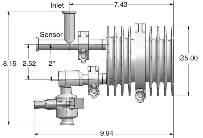
Vertical Inlet, No Sensor, One-body Segment, Model SSC-075-VN1...
