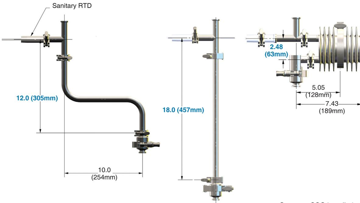
Typical 18" lineal, 12" vertical (bent tube) downcomer assembly
