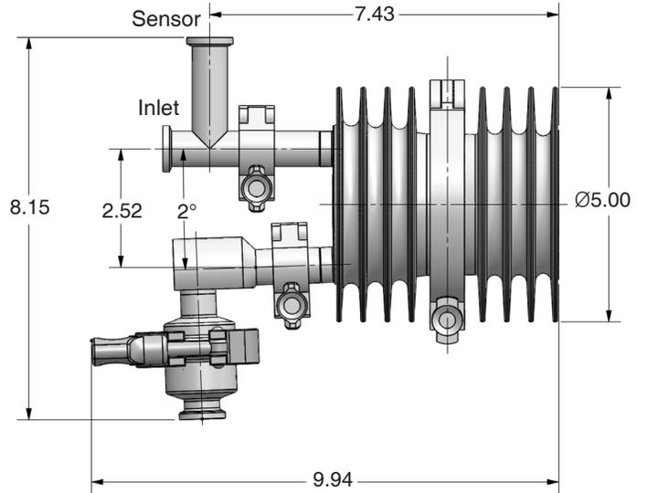
Horizontal Inlet, No Sensor, One-body Segment,
