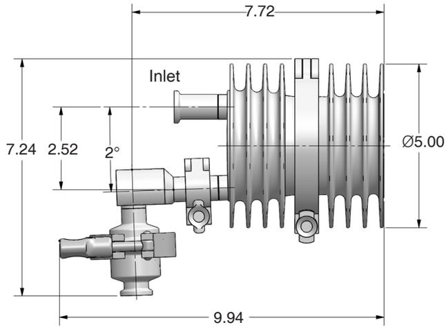
Horizontal Inlet, Sensor, Two-body Segments,
