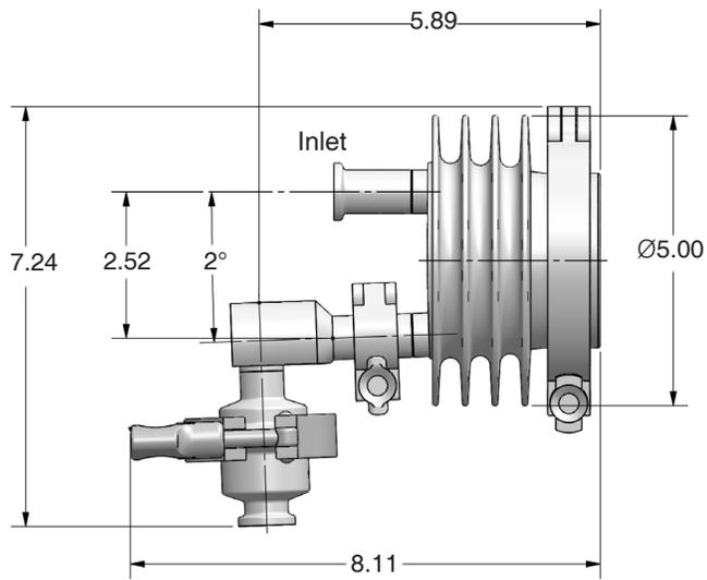
Horizontal Inlet, Sensor, One-body Segment,
