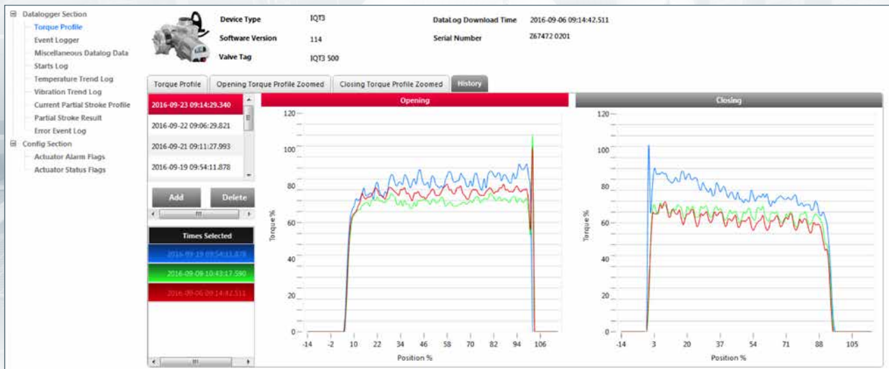
Above: Rotork's intelligent asset management system showing torque data from multiple actuator datalogs.
