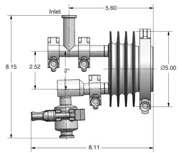
Vertical Inlet, Sensor, One-body Segment, Model SSC-075-VS1...
