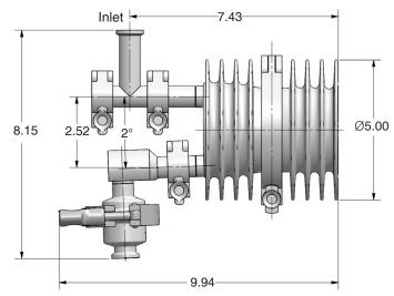
Vertical Inlet, No Sensor, Two-body Segments, Model SSC-075-VN2... Vertical Inlet, Sensor, Two-body Segments, Model SSC-075-VS2...
