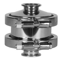
The Mark 934 is designed to operate up to a maximum differential pressure of 50 psig (3,4 bar) and will control condensate subcooling to less than 5°F, over a range from 10 to 50 psig.
